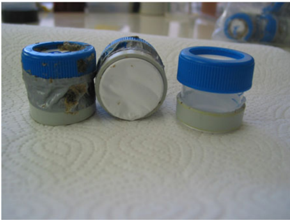
Fig. 2 Carriers for introduction of composting substrate contaminated with C. m. ssp. sepedonicus into sanitation processes
