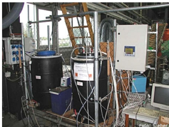
Fig. 1 Composters (60 l) used for experiments in a quarantine station
